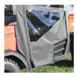
10. To open and stow the doors, move the zipper fully rearward and fold the bottom portion of the doors up. Then begin to form a vertical roll with the door by rolling it inward from the front edge toward the rear of the door. Secure in place using the two hook and loop straps provided. Try to form a roll approximately 2" in diameter to assure that the door will not stick out very far while stowed.
