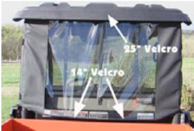
6. You will see six 8" adhesive Velcro strips with the cab. These will be attached to the inside of the windshield down the sides. Three pieces per side have been supplied because it is a curved piece of metal and the adhesive Velcro does not curve well. The photo below shows where to attach these.
